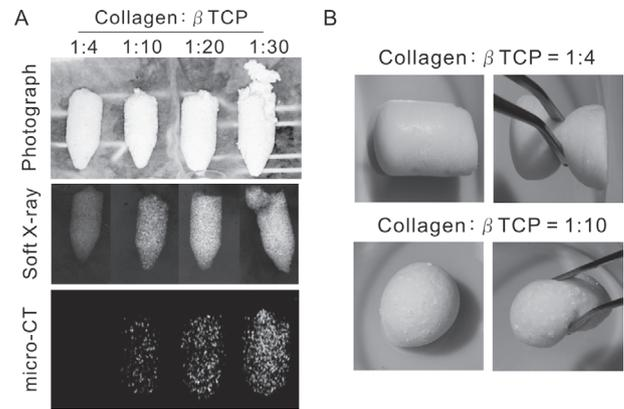
**Fig. 1** (A) Photographs, soft X-ray and micro-CT images of the beta-tricalcium phosphate ( $\beta$ -TCP)-collagen composite materials with various  $\beta$ -TCP particle-to-collagen ratios. Shown is the structural collapse of composites with  $\beta$ -TCP particle-collagen ratios of 20 : 1 and 30 : 1. (B) Photographs of  $\beta$ -TCP-collagen composite materials with  $\beta$ -TCP particle-to-collagen ratios of 4 : 1 and 10 : 1 were pinched with forceps exerting equal force.
