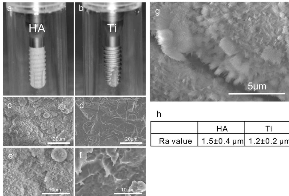
**Fig. 1 – Photographs of scanning electron microscopic images nanopolymorphic crystalline HA-coated (a, c, e and g) or anodic oxidized (b, d and f) implants. Arithmetic mean estimation (Ra) values measured with laser microscopy are no significant difference between both types of implants (h).**
